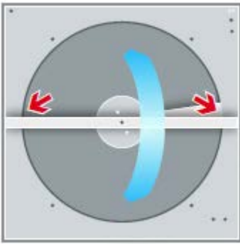
Figure 6 The arrows indicate the measuring points. The blue line indicates the inclination.
