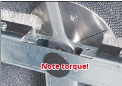
Figure 4 When the rotor is positioned at a suitable angle, tighten the hex head screw to the correct torque.
