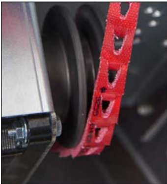
Figure 7.4.4.1: The belt direction is marked on the belt with an arrow.
