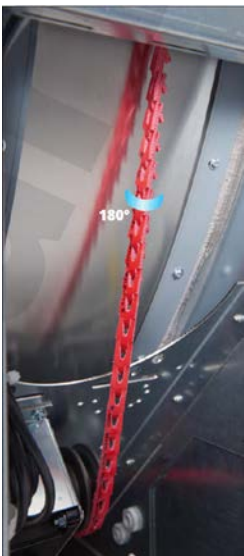
Figure 7.4.4.2: Ensure that the belt rotates around the motor pulley and rotor as shown. After installation, the belt rotates 180 degrees as the rotor rotates.
